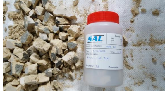
MPS 20: Sample of bricks collected from Chimney 4 at the start of demolition of the upper part of the chimney
